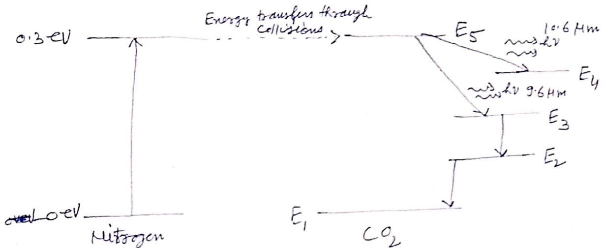
Fig. - Energy levels of CO<sub>2</sub> & N<sub>2</sub> molecules and transitions
