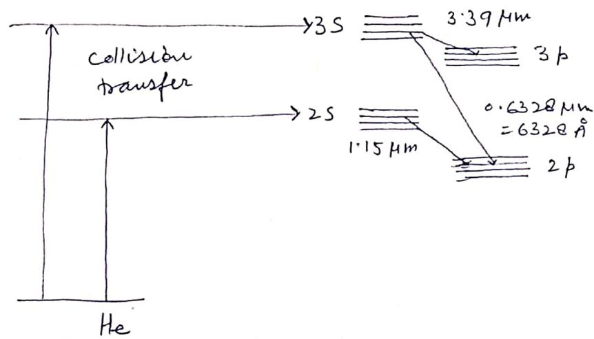
Fig. - Partial energy level of He-He gas LASER.
