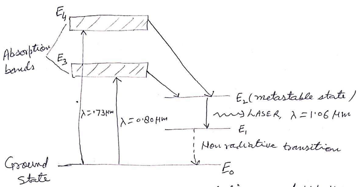
Fig. - Energy level diagram of Nd:YAG LASER.
