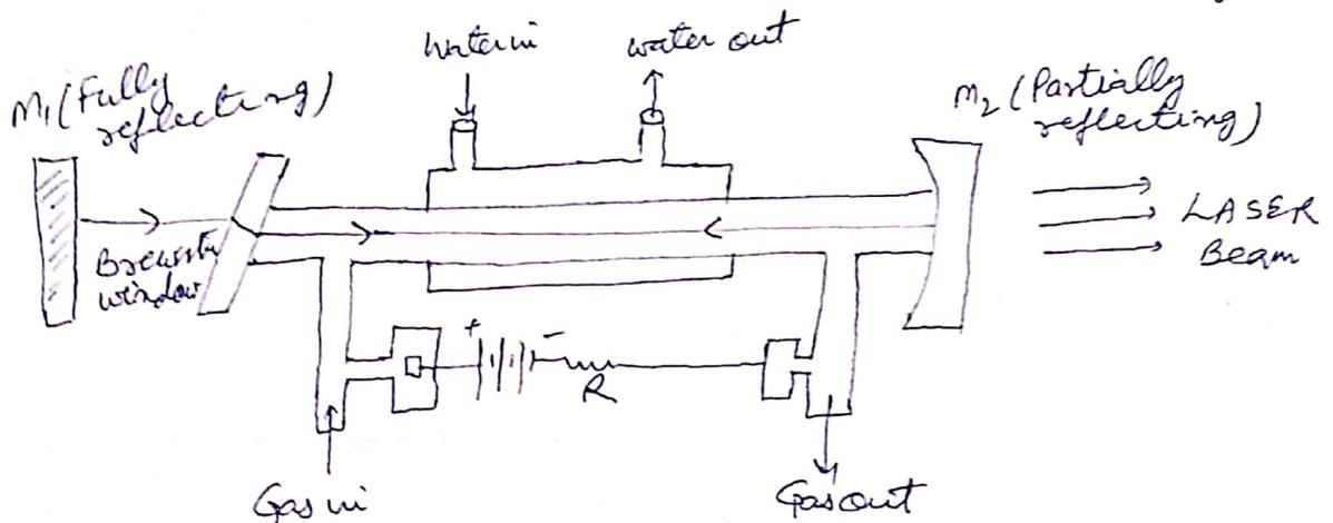
Fig. - A schematic of typical  $\text{CO}_2$  LASER.
