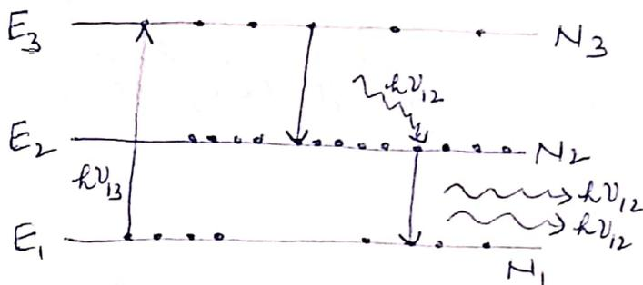
Fig. - optical pumping
