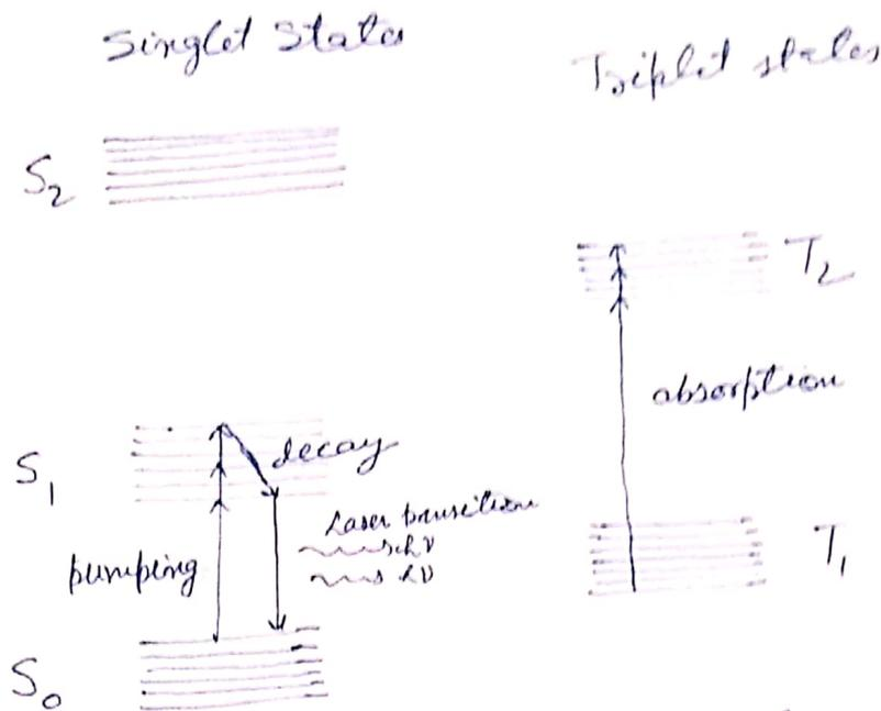
Fig. - Schematic representation of the energy levels of an organic dye molecule.
