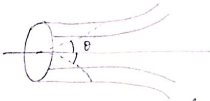
fig - Directionality of laser beam
