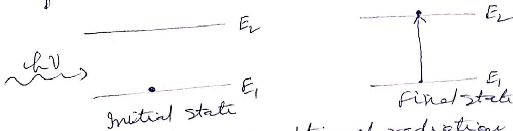
Fig. - Absorption of radiation
